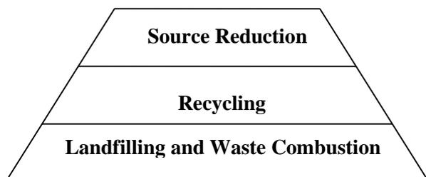
**Figure 6.** Integrated solid waste management hierarchy
