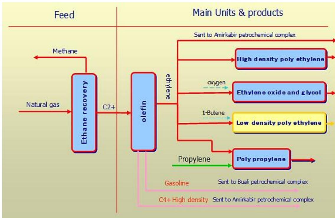
Figure 2. Brief process diagram of Marun petrochemical complex
