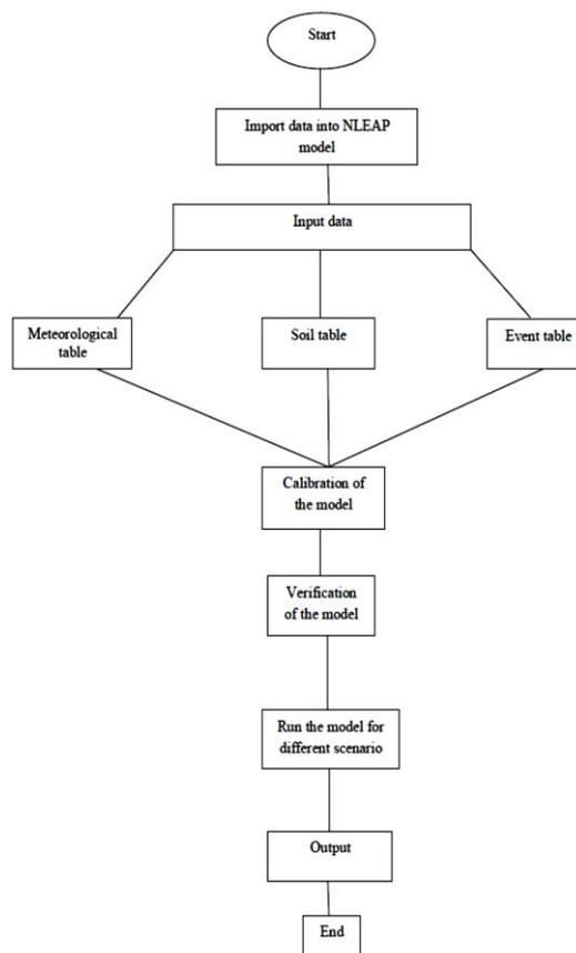
Figure 2. Flowchart of the NLEAP model
