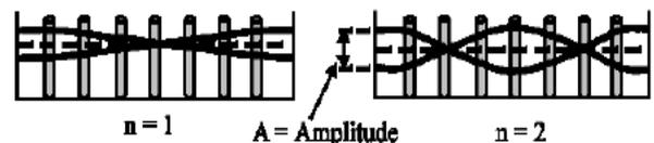
**Figure 2.** Modes of waves appearing in the laboratory flume
