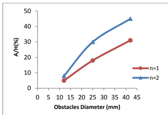
Figure 4. The variations of A/H against obstacles diameter
