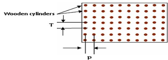
**Figure 1.** In-line arrangement of the wooden cylinders
