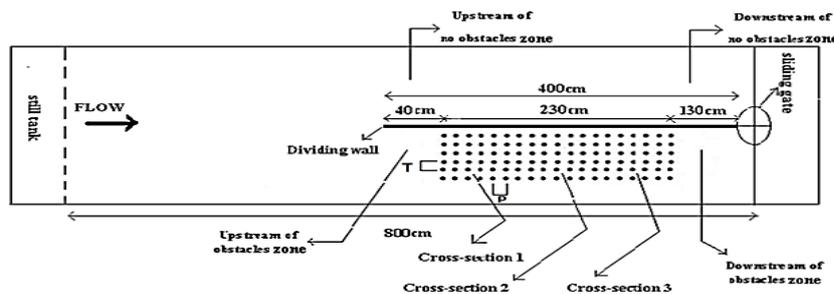
Figure 3. Specifications of experimental flume
